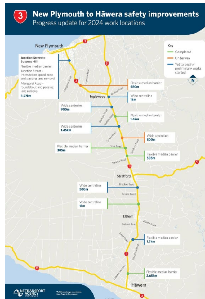
Figure 11 – New Plymouth to Hāwera Safety Improvements
