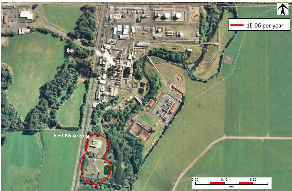
Figure 7-5: 1E-06 per year Risk Contour Contributed by the LPG Storage & Loadout Area Scenarios only
